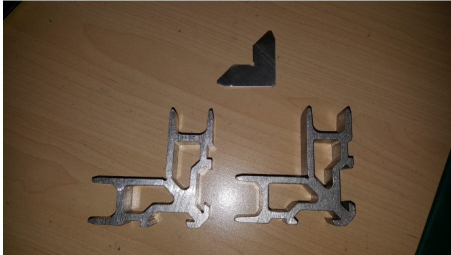
Corner Bracket Inserts – Main Frame
