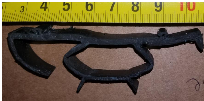
Interior side frame gasket for the sill
