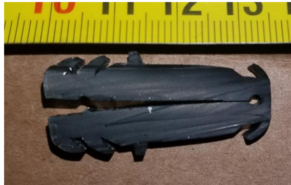
Gasket joining the frame profiles for the sill and the vertical mullions
