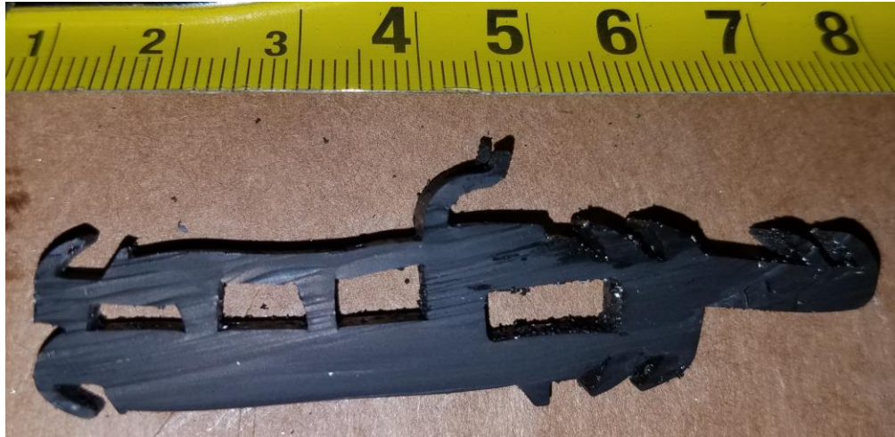
Gasket joining the main frame and sub frame profiles for the sill.
