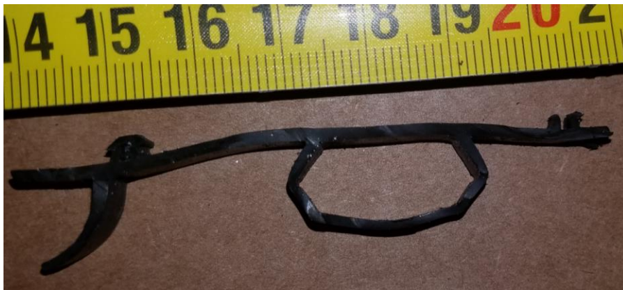
Interior side frame and sub frame gasket for the jambs
