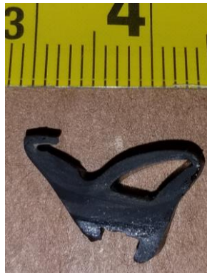
Glazing stop side glazing gasket
